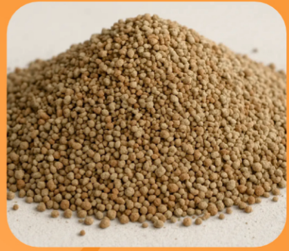
Boiler Bed Material
